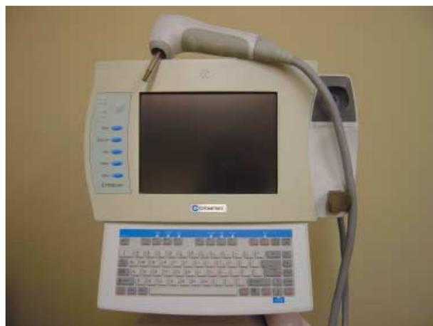
**Figure 3** Portable device that allows the inspection of individual capillaries of the cutaneous microcirculation and flow through these vessels in real time. Cytoscan<sup>®</sup> by Cytometrics<sup>®</sup>. (Courtesy of Laboratory for Research in Microcirculation, Universidade do Estado do Rio de Janeiro, Rio de Janeiro, Brazil)
